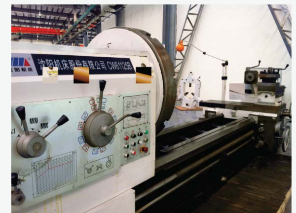
CW61125 Horizontal Lathe with Max. Machining Diameter of 8 m
