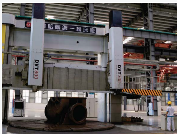
DVT800 CNC Vertical Lathe with Max. Machining Diameter of 8 m
